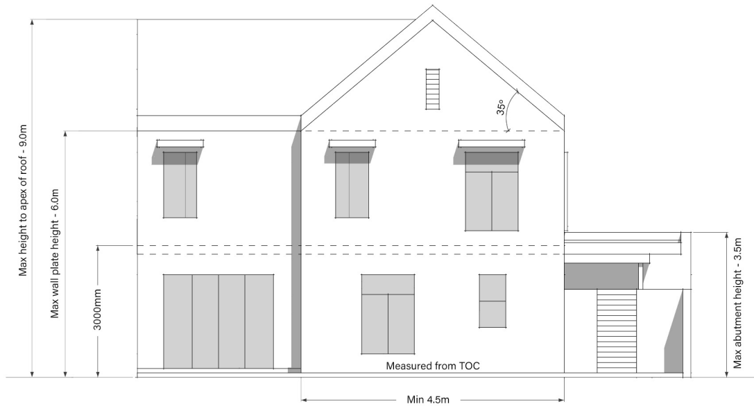
Figure 27: Illustration of the building heights associated with a typical double storey building
